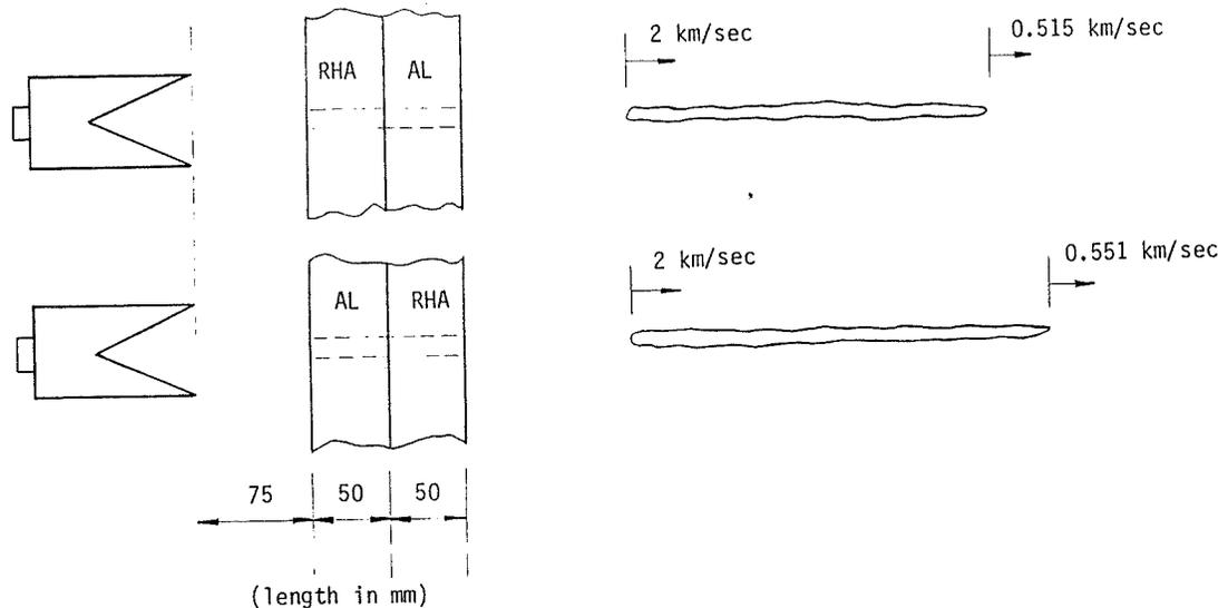
Figure 5. Schematic Showing Residual Jet Length and Velocity of a Copper Jet with Initial Tip Velocity of 10 km/sec after Perforating an RHA-Aluminum, and an Aluminum-RHA Plates.
